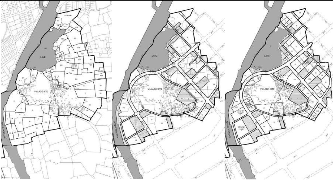
Figure 7: Identification & Inventory of all parcels, planning roads and amenities, readjustments of parcels in proportion to original holdings
