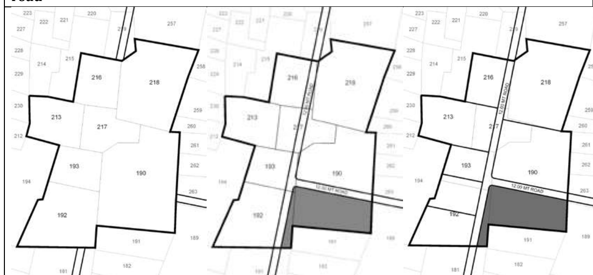
Figure 6: Land Parcels before the road, with the road & after readjustments around the road
